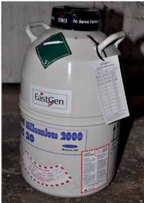
Liquid nitrogen tank
